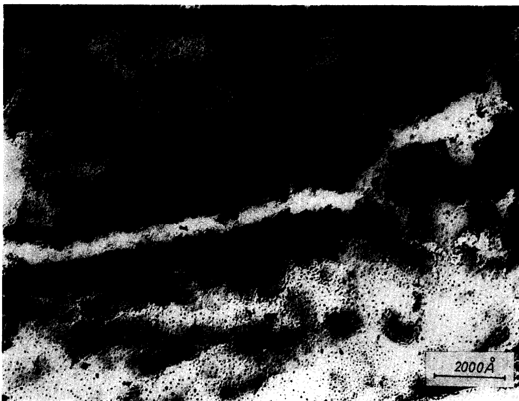
FIG. 4. Transmission electron micrograph after the model catalyst from Fig. 3 was annealed in air at 500°C for 24 hr and slowly cooled to room temperature. The average size of the metal crystallites is 39 Å.
